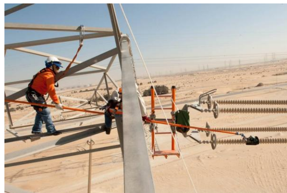
Composite Insulator Testing using the Electric Field Method
