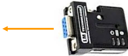
Ensure the slide switch on the Bluetooth adapter is in the DCE position.
