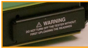
Locate Power Switch Cover and remove
