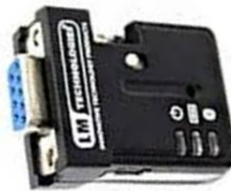
Ensure the slide switch on the Bluetooth adapter is in the DCE position.
