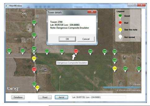
The next click opens the information table for the insulators of that tower. Choose an insulator and then click on **Graphic**. The associated graph of the E-Field of that insulator is displayed clearly showing the defect. Click on **Tower Picture** to see the picture of the associated tower.
