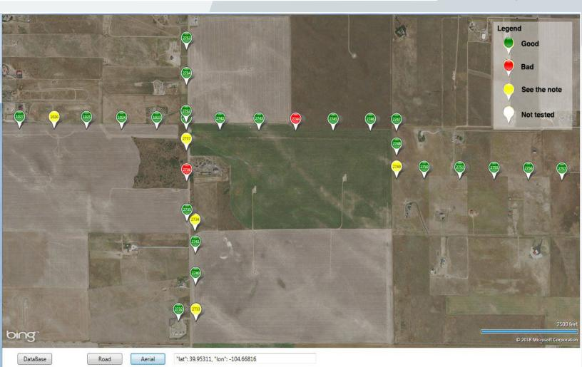
Positron's Mapping System displays at a glance the health and location of the insulators in the power network. Using a JSON database from Positron's Insulator Testers, it includes the tower identity, its GPS coordinates, the condition of the insulators identified by line, phase, etc. and supplemental data that the power utility can tag to each tower, Color-coded tags show you where
